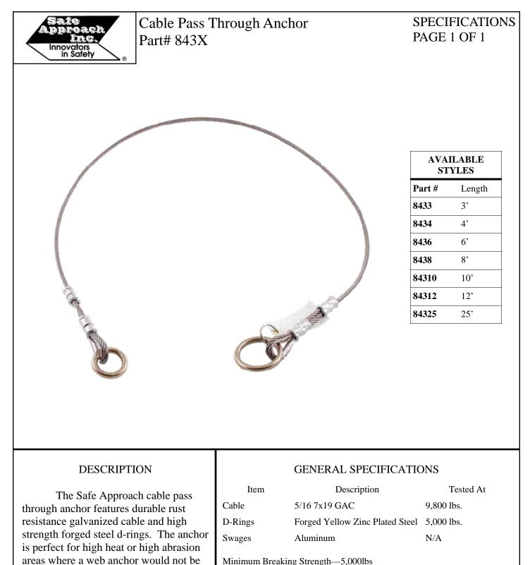
Minimum Breaking Strength—5,000lbs Capacity—1 Worker, Max Total Weight 400lbs
